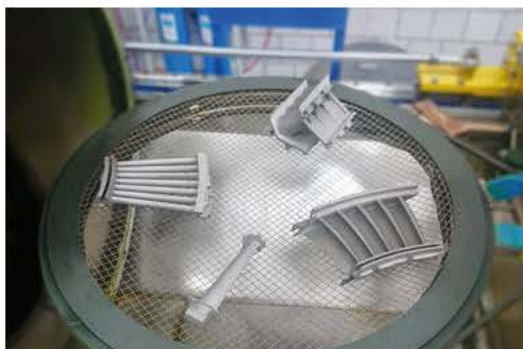
KAMA system: rotating table. Loading/Unloading of inspected objects
