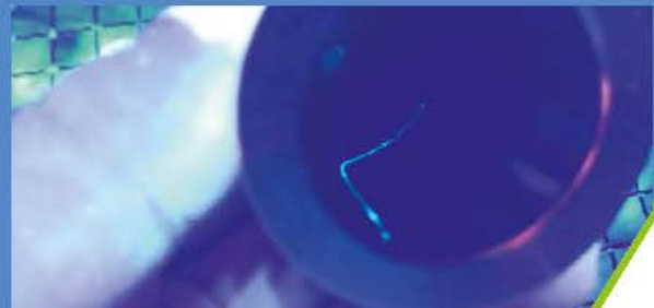
Nozzle. Titanium alloy. A long crack on the inner surface
