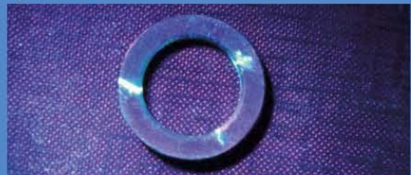
Disc. Through radial cracks
