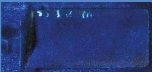
Blade of titanium alloy with multiple linear indications of defects such as cracks
